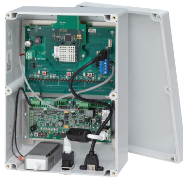
Photo shows AC-ALL-SCH-PIM400-1501-LC panel interface module with AC-MER-CONT-1DR Mercury EP1501 controller
